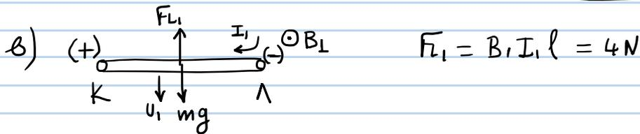
$$\frac{dE_{\text{Mech}}}{dt} = \frac{dK}{dt} + \frac{dU}{dt} = \Sigma F \cdot v_1 - mg v_1 = (mg - F_{L1}) v_1 - mg v_1$$
