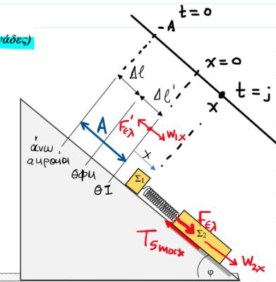
$$\text{οπως } T_{\text{max}} = \mu_s N_2 = \mu_s m_2 g \mu \varphi = \frac{\sqrt{3}}{2} 80 \cdot \frac{\sqrt{3}}{2} \Rightarrow T_{\text{max}} = 60 \text{ N}$$
