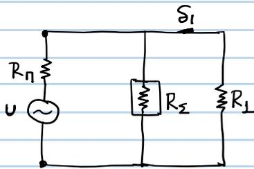
$$R_1 // R_2 : R_{12} = \frac{R_1 R_2}{R_1 + R_2} = 1 \Omega \quad R_{\text{ολ}} = R_1 + R_{12} = 4 \Omega$$
