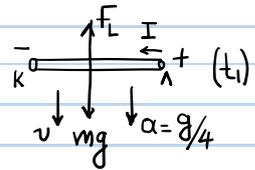
$\Sigma F = ma \Rightarrow mg - F_L = \frac{1}{4} mg \Rightarrow F_L = \frac{3}{4} mg$
