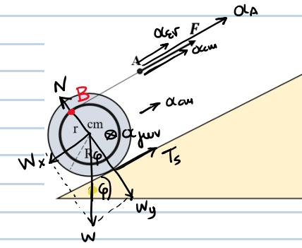
$$\text{οπως } r \alpha_{fpr} = \frac{4}{5} R \alpha_{fpr} = \frac{4}{5} \alpha_{cm} \quad \text{αφα } \alpha_A = \alpha_{cm} + \frac{4}{5} \alpha_{cm} = \left(5 + \frac{4}{5} \cdot 5\right) \omega / s^2 \Rightarrow \alpha_A = 9 \text{ rad/s}^2$$
