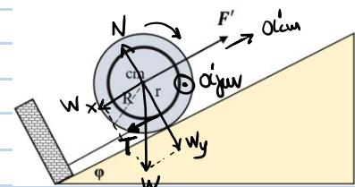
$$\Theta \text{ΝΣ: } \sum T' = I_{cm} \alpha'_{fpr} \Rightarrow T_T = I_{cm} \alpha'_{fpr} \Rightarrow T \cdot \nu = \frac{1}{2} m R^2 \alpha'_{cm} \Rightarrow T = \frac{1}{2} m \frac{R^2}{0,64 R} \alpha'_{cm} \Rightarrow T = \frac{m \alpha'_{cm}}{1,28}$$
