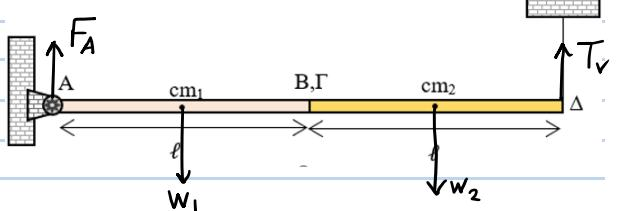
$$\sum T_A = 0 \Rightarrow T_{T_v} - T_{w_1} - T_{w_2} = 0 \Rightarrow T_v 2l - w_1 \frac{l}{2} - w_2 \frac{3l}{2} = 0$$
