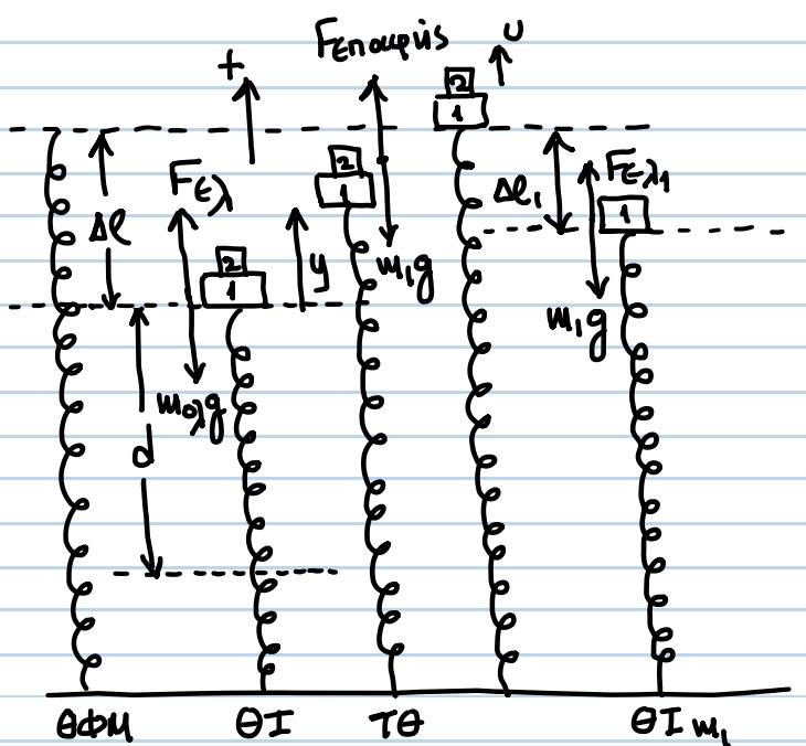
$$\sum F_2 = m_2 \alpha \Rightarrow F_{\text{ηελαφρής}} - m_2 g = -m_2 \omega^2 y \Rightarrow F_{\text{ηελαφρής}} = m_2 g - m_2 \omega^2 y$$
